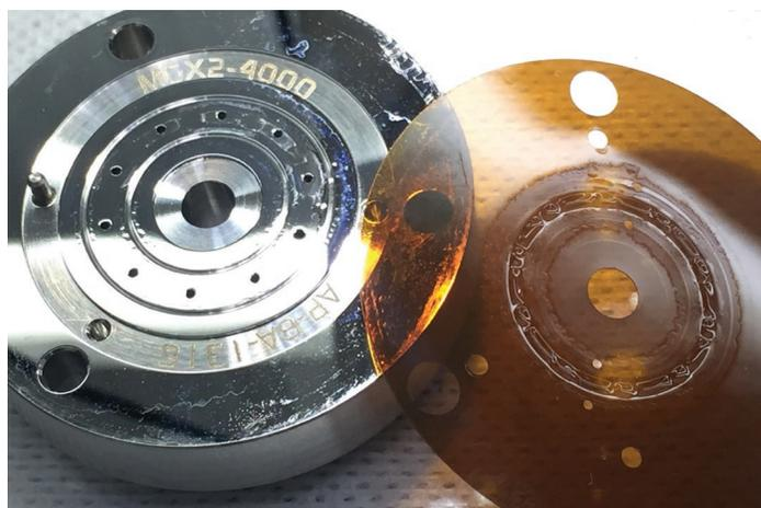
**FIGURE 1 :** Valve head contamination
