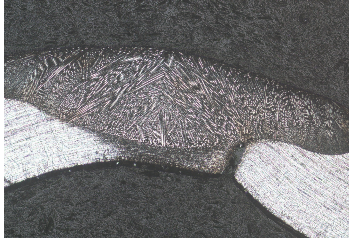
FIGURE 1 : Misaligned strip edges create an off-seam condition and incomplete penetration.
